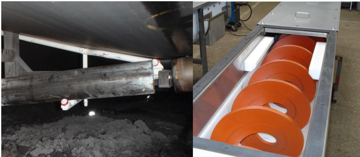
Duromer FRAS-approved materials replace metals in surface and sub-surface applications, including underground conveyor rollers, left
